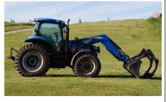
raised, the tractor's center of gravity is raised and moved forward. The tractor's stability is reduced; thus, increasing the chance of overturning.
