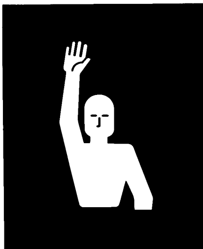
Figure 5 —STOP—Raise hand upward to the full extent of the arm, palm to the front. Hold that position until the signal is understood.
