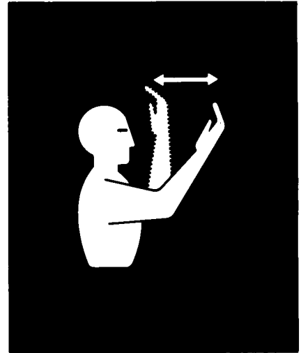
Figure 3 —MOVE TOWARD ME—FOLLOW—ME Point toward person(s), vehicle(s), or unit(s), beckon by holding the arm horizontally to the front, palm up, and motioning toward the body.
